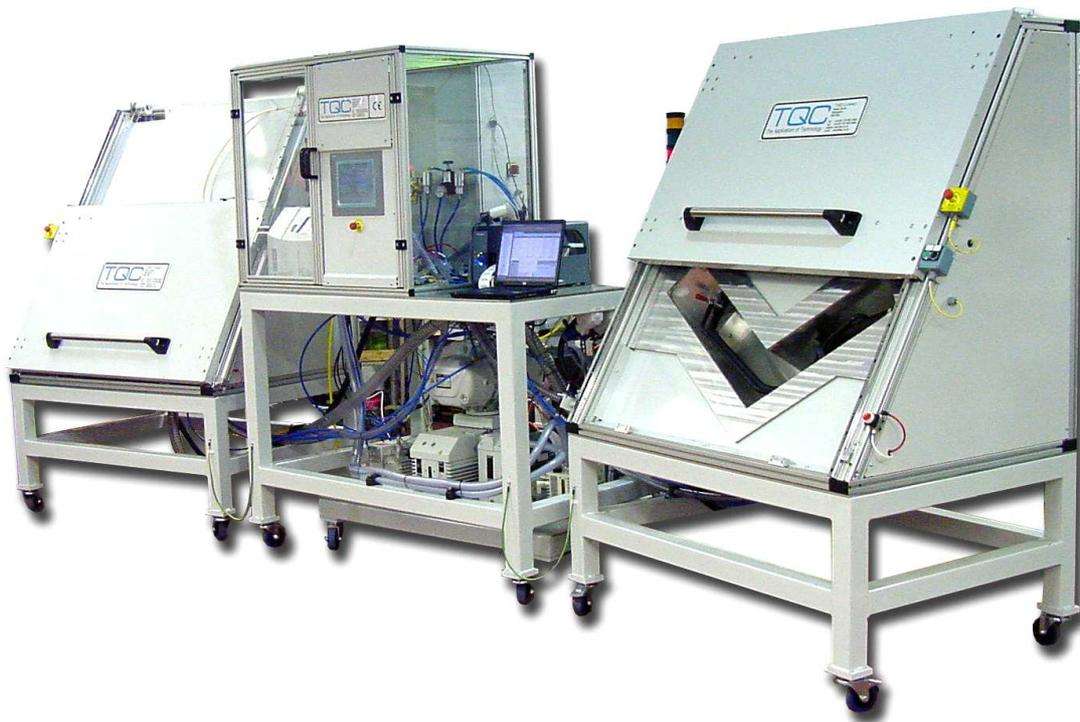
TQC designed and manufactured 2 helium leak test systems for the automatic testing of plastic fuel pipes. The systems included bespoke tooling to accommodate 2 variants of fuel pipe.
